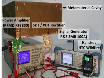
Fig.4 Measurement setup of wireless charging system of mobile handset.
