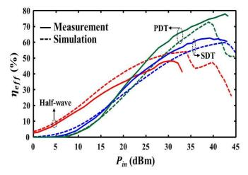
Fig. 3 Measured and simulated  $\eta_{e\!f\!f}$  of SDT and PDT rectifiers versus  $P_{in}$  .
