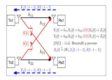
Figure 1. Two-user bursty interference channel
