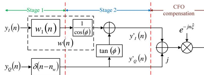
Figure 2: Compensation structure
