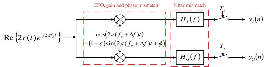
Figure 1: Structure of wideband direct-conversion receivers
