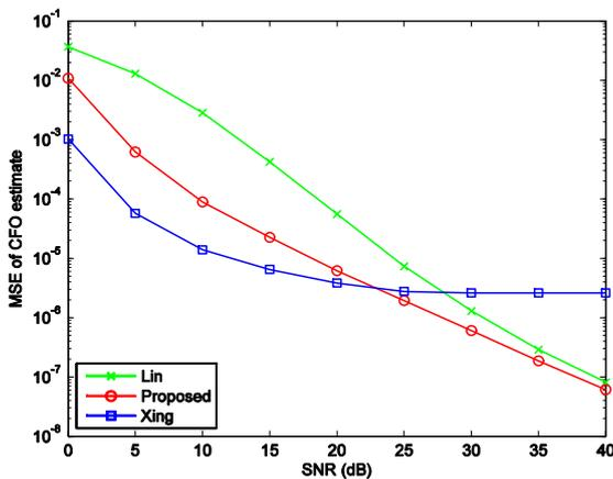
Figure 3: MSE of CFO estimate versus SNR
