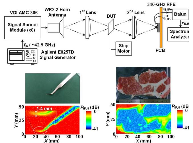
Fig. 4. Proposed THz transmissive imaging system.
