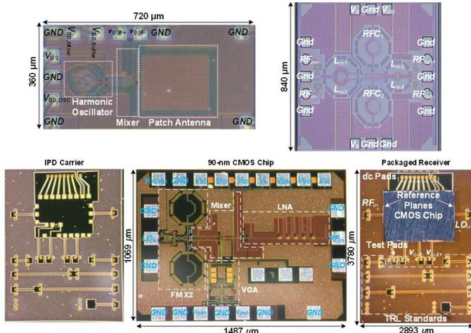
Fig. 3. Proposed THz receiver, V-band frequency doubler, and W-band packaged receiver.
