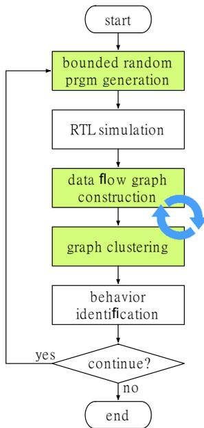
Fig. 2 The test program template generation flow.
