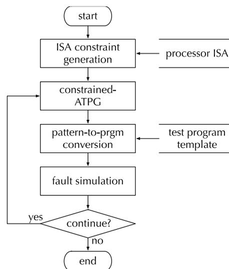
Fig. 1 The self-test program generation flow.
