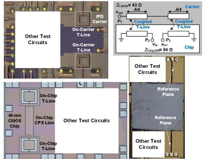
Fig. 2. Proposed balun-embedded THz interconnect.
