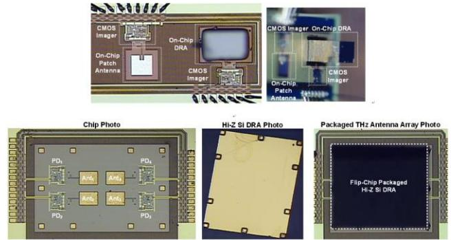
Fig. 1. Proposed THz dielectric resonator antennas.
