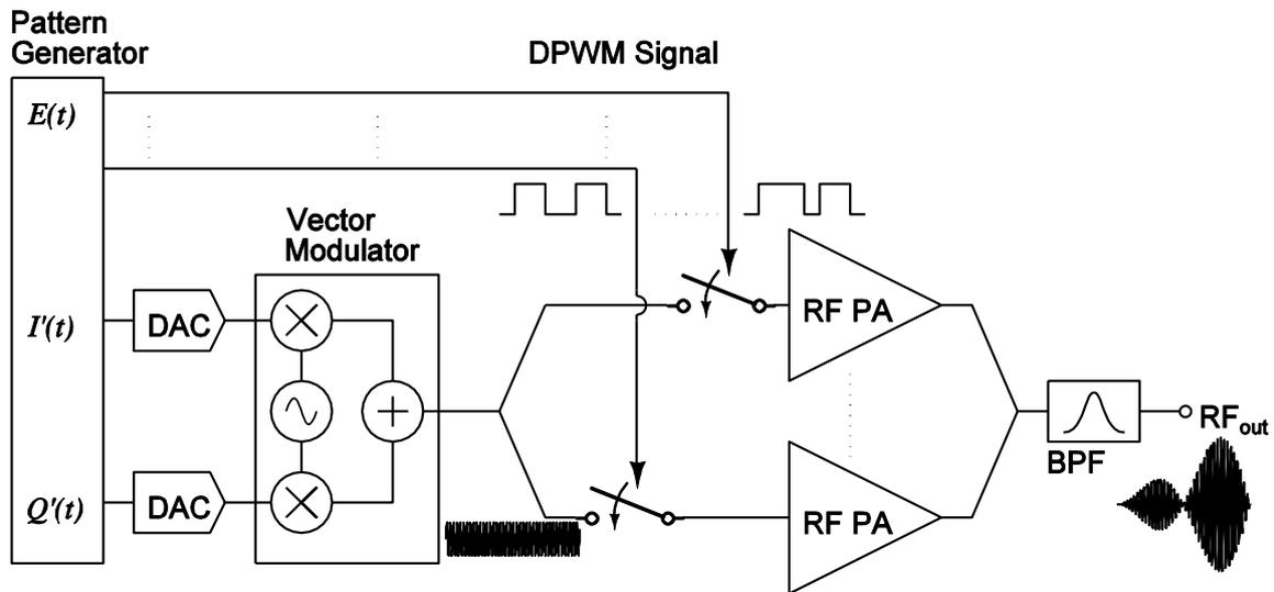
Fig. 1. Schematic diagram of a dual-level pulse modulated polar transmitter.
