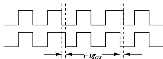
Fig. 2. Example of a dual-level DPWM signal.
