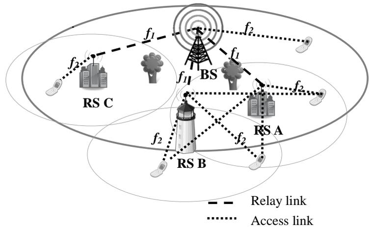
Fig 1. An example of RS cooperation in a wireless relay network.
