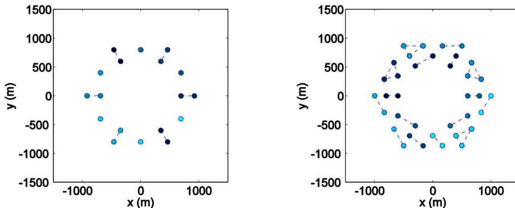
Fig. 4. Strategic RS placements. Left: 18 RSs, two-tier topology. Throughput gain = 1.3596. Right: 36 RSs, three-tier topology, throughput gain = 1.476
