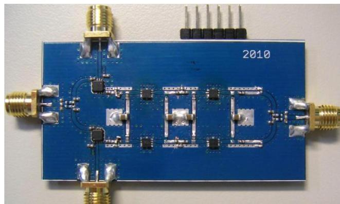
Fig. 3. Prototype of the dual-level pulse modulated polar transmitter.
