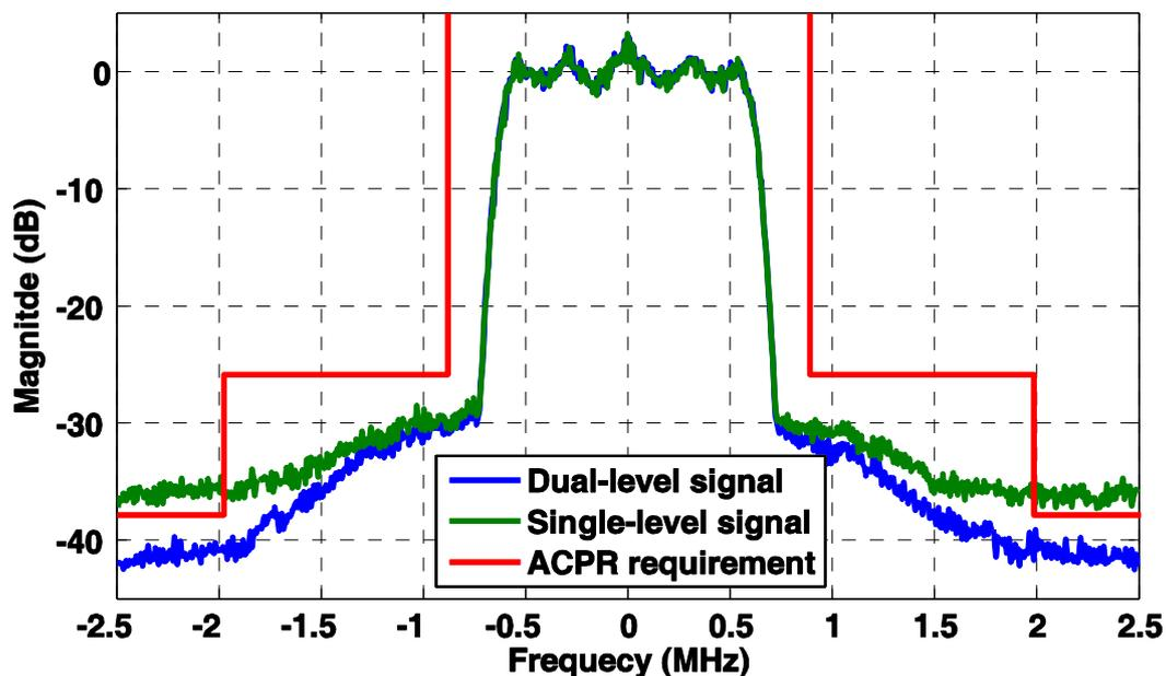
Fig. 4. Comparison of the output spectrums of the pulse modulated polar transmitter using a dual-level signal and a single level signal centered at 836.5 MHz.
