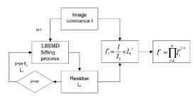
Fig. 5 The processing flow diagram of LBEMD for natural color/gray-level images.
