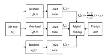
Fig. 9 The processing flow diagram for proposed color constancy method.
