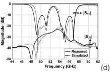
Fig. 5. (a) LTCC single-branch laminated waveguide diplexer. (b) Traditional and proposed coupling structures. (c) Insertion loss, (d) return loss, and isolation of the diplexer.
