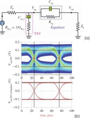
Fig. 4. (a) Simplified TSV model after significant analysis with proposed RC equalizer. (b) Eye diagrams before and after compensation.
