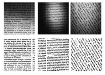
Fig. 3 First row: Text images with uneven illumination. Second row: Uneven illumination removal with proposed LBEMD method.
