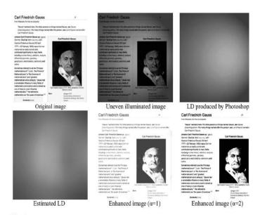
Fig. 4 Original image, uneven illuminated image, LD produced by Photoshop, estimated LD, a enhanced images by LBEMD. Peak signal-to-noise ratio (PSNR) is 17.03 dB for  $\alpha = 1$  and 19.99 for  $\alpha = 2$ .
