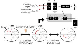
Flow charts of matching network synthesis. Each Fig. 1 unknown block (symbol '?') is one of the distributed components. The [ai, bi] and [ci, di] denote the range of EL and Z<sub>0</sub> which belong to component i respectively.
