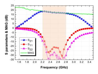
Fig. 5 The S-parameters of matched NE-42484, which is matched with global optima of  $\Gamma_{MS}(f)$  and  $\Gamma_{ML}(f)$ . It is obvious that the  $|S_{21}|$  dB is almost the same of MAG in 2.2-2.8 GHz (highlight) due to optimized matching.
