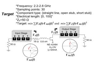
Fig. 3 The example for performance measurement of our proposed algorithm. The synthesis target is to employ 4<sup>th</sup>-order network to synthesize broadband simultaneous-conjugatematching from 2.2 to 2.8 GHz. The gate of the transistor is connected with small resistor to ensure the existence of simultaneous-conjugate-matching condition, and the effective series inductance (ESL) is also considered.
