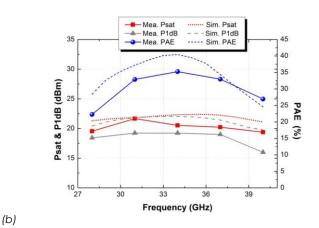
Fig. 9 (a) Measurement and simulation results of S-parameter from 1 GHz to 50 GHz. Both the in-band gain and return loss are desirable due to good synthesized matching. (b) Frequency response of large signal. The P<sub>sat</sub> is 22 dBm with 33% peak PAE at 31 GHz.
