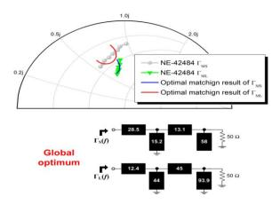
Fig. 4 The curves of  $\Gamma_{MS}(f)$  and  $\Gamma_{ML}(f)$  of stabilized NE-42484 transistor, and the correspondent frequency response (solid line without symbol) and circuit topology of optimal matching network are also illustrated.
