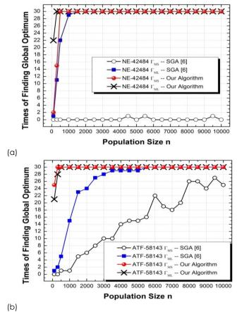
Fig. 6 (a) The times of finding global optimum in matching  $\Gamma_{MS}(f)$  and  $\Gamma_{ML}(f)$  of transistor NE-42484. (b) Statistic for transistor ATF-58143. The function evaluations of algorithms are 100n. Since the [6] is not robust algorithm, which usually takeover by other local optima; while our algorithm can find global optimum with 100% statistic probability when n is larger than 500.
