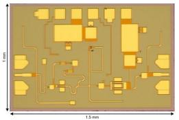
Fig. 8 Chip photograph with a compact chip size 1×1.5 mm2.
