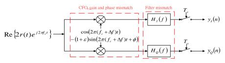
Figure 1: Structure of wideband direct-conversion receivers
