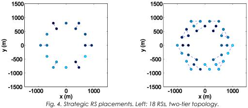
Throughput gain = 1.3596. Right: 36 RSs, three-tier topology, throughput gain = 1.476
