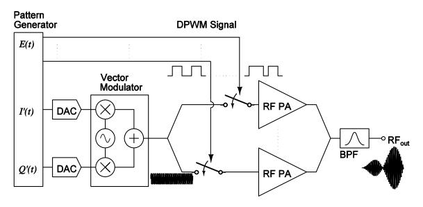
Fig. 1. Schematic diagram of a dual-level pulse modulated polar transmitter.
